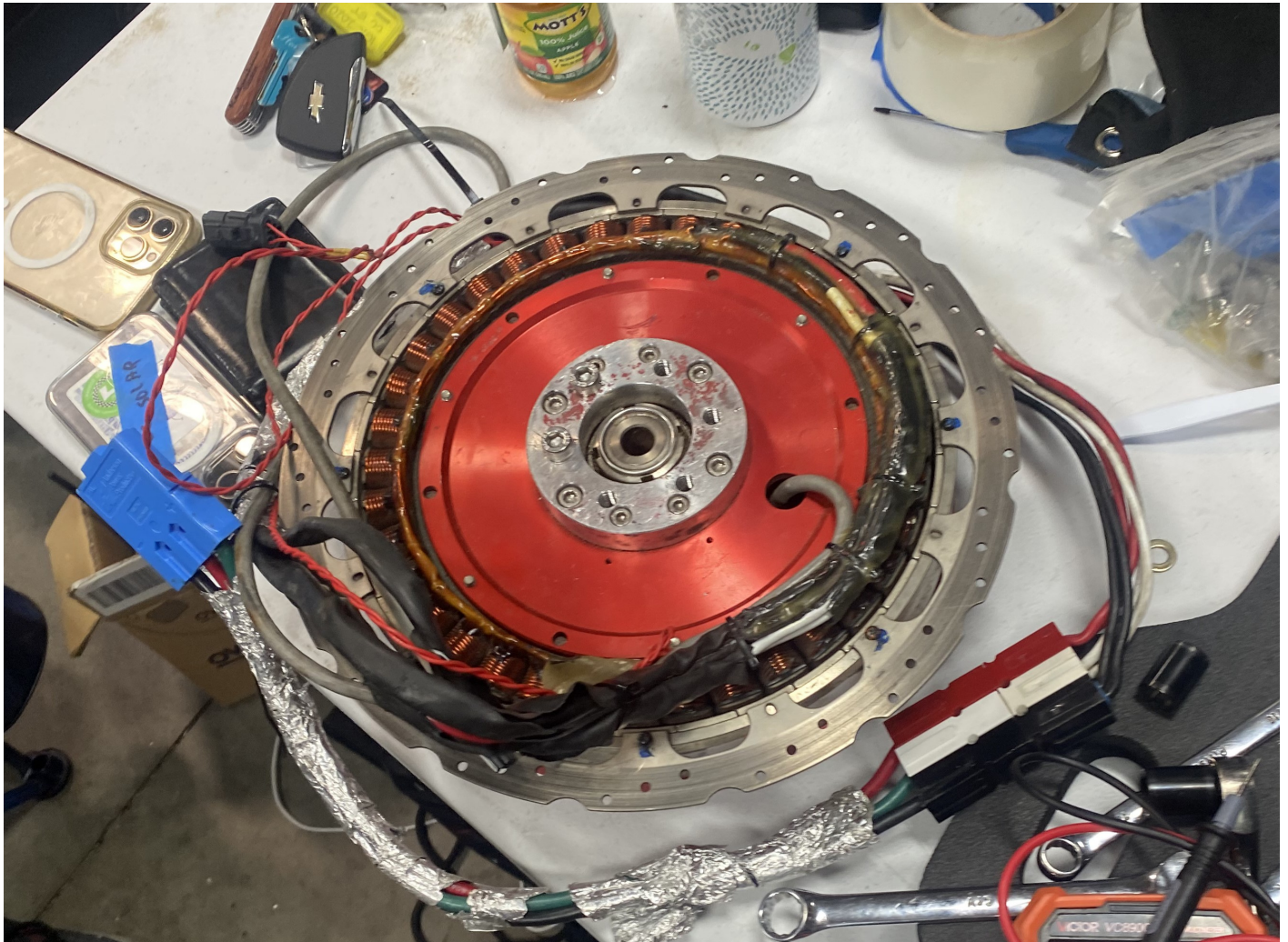
(Figure 3) Notice the copper wire coils as part of the stationary element (stator) and the metal outer rotating element (rotor). Notice that the motor power wires enter the stator.
